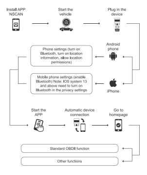
3.3 Turn on Bluetooth- Start the app- Automatic connection will be built - Connected.
